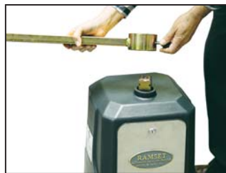
4. Carefully lift off the clamp release and arm.
