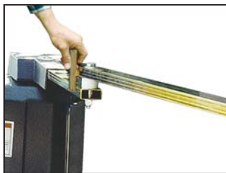
3. Slightly bend the arms at the elbow and secure the gate from free-movement to relieve the pressure on the operator from the gate.
