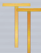
Post Mounts 1/4" angle iron flats. 3/16" square tubing legs. Used to mount the operator off the ground.
