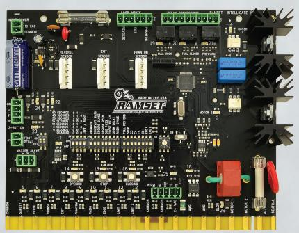
The Intelligate control board is the most advanced gate controller in the industry, putting Ramset ahead of the competition when it comes to reliability and number of features. It is controlled by a programmable microprocessor that reads and precisely executes all functions of the control board. Some of the features of the control board:
