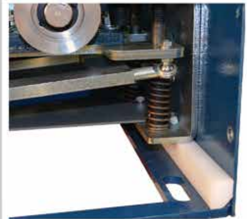
Spring mounted suspension that moves with rail
